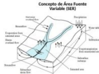
Figure 2. Conceptual description of the hydrological processes included in a simple model.
